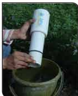
Clean Threads with Water before joining
